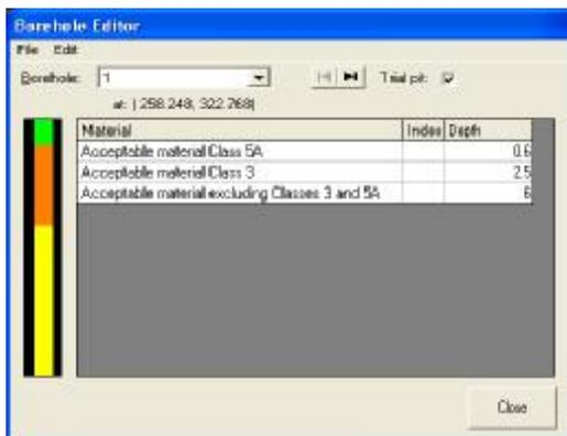
Boreholes can now be set as Boreholes or trial pits, the only difference being trial pits are drawn square and boreholes circular.
