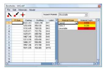
Once boreholes have been entered and materials and depths associated with each one it is possible to view the borehole triangles from the standard show menu and dynamic sections has an option to view borehole materials.
