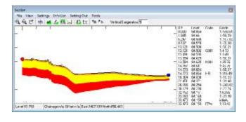
The depths of materials are entered as if they are measured continuously from the ground level to the underside of each material. i.e. they are the accumulative depths
