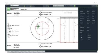
This is a stand alone tool that compares a set of surveyed points against factory set targets on the machine giving the roll, pitch and yaw in relation to the proposed alignment
