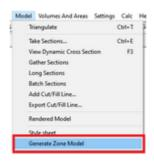
You can then populate start and end chainages, max and min offsets for each zone along with an interval for it to add points on the edge of the model
